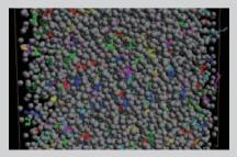
A computer simulation showing a molecular-level view of the principal constituents of tires (gray: silica particles;\* color: partially rendered polymers)
