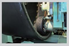
Inside-Drum Testing Machine A machine that monitors the key performance metrics of tires when cornering on dry, wet or icy roads
