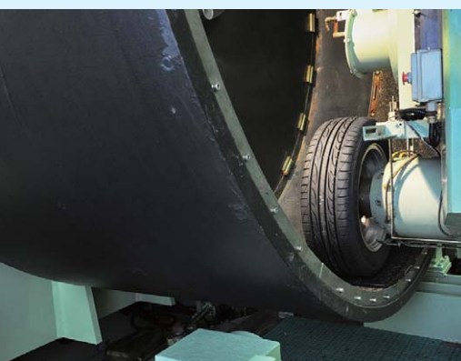
Inside-Drum Testing Machine A machine that monitors the key performance metrics of tires when cornering on dry, wet or icy roads
