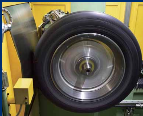
A rolling resistance testing machine
